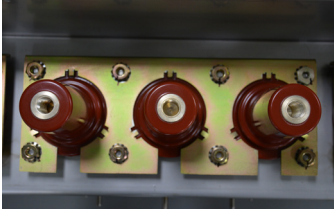
C / V : plug-in bushing NF EN 50181, with C type connection (Ir: 630 A; Ø M16 mm)
